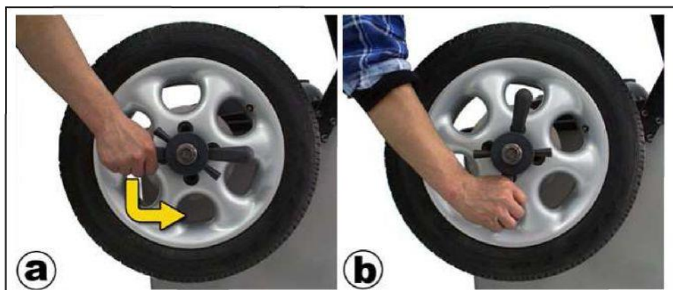
Fig. 5.8 Dismounting the wheel from the holder.
