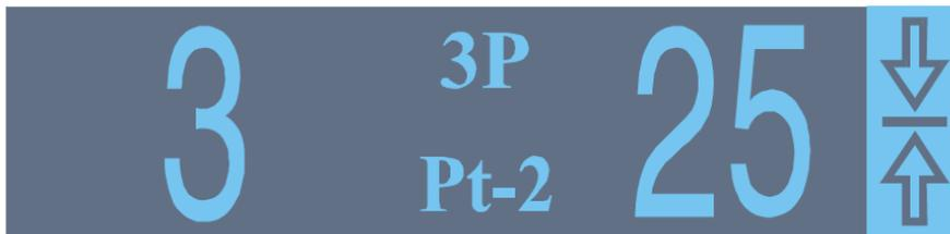
It is a position in which the correction weight of 25 g should be stuck.
