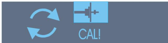
4. Spin the shaft so as to reach the rotational speed of 125 rpm. Calibration cycle starts when the shaft revolutions are brought up to speed of 125 rpm.
